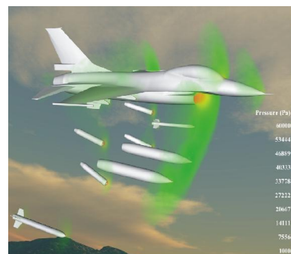
Simulation of an F16 aircraft store separation case.
